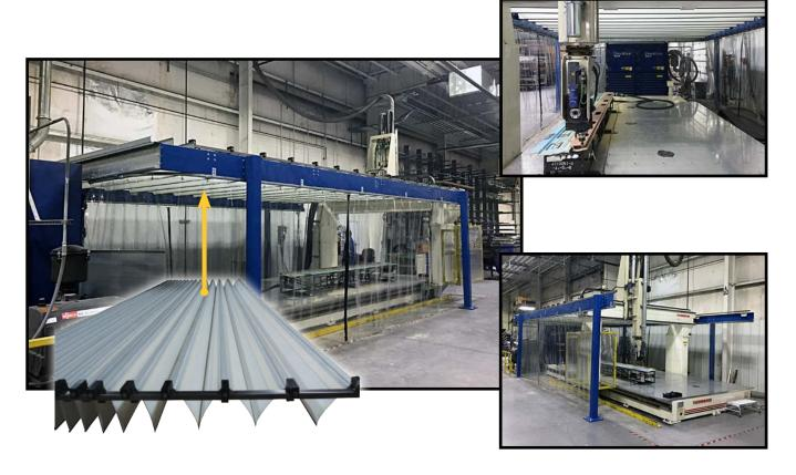
Dynatect's retractable machine roof cover contains debris and noise during machining of large aerospace parts. The translucent cover material allows light to enter.
